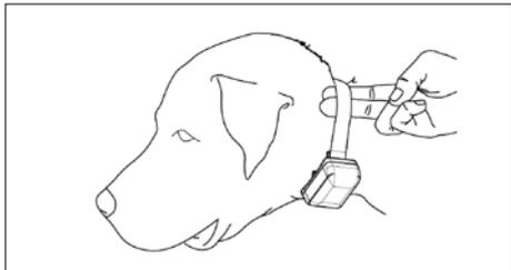
The collar should be fitted so that the Surgical Stainless Steel contact points press firmly against the dog's skin. You should be able to fit a finger in between the contact point and your dog's skin.
