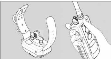
1. To activate your Dogtra 3500NCP Super-X Series place the red dot on the back of the transmitter to the red dot on the receiver/collar. Hold the two red dots together for a moment until the green colored LED indicator light comes on.
