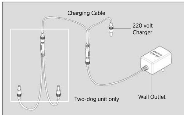
The battery charger and charging cables allow you to charge both the transmitter and receiver at the same time. The battery charger is designed for a 220-volt wall outlet (U.S.A. 110-volt AC chargers and 10-volt field charger for Lithium-Polymer batteries for your automobile are also available.).
