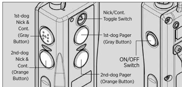
The Dogtra 3500NCP Super-X Series has five buttons and a toggle switch on the transmitter. Two on the face of the transmitter, two on the left side, and one on the right side.
