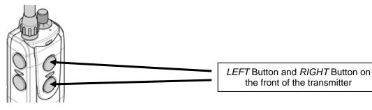
3. Hold the *LEFT* button and the *RIGHT* button on the front of the transmitter simultaneously down for 3 seconds or until the rapid green blink of the LED on the receiver resumes a slower pace. The code setting work is now completed.
