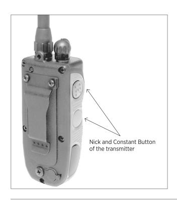
Hold the Nick button and the Constant button on the left side of the transmitter simultaneously down for 3 seconds or until the rapid green blink of the LED on the receiver/collar resumes a slower pace.
