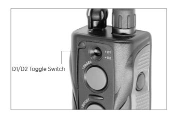
Start with the receiver/collar turned off and the transmitter turned on. On the front of the transmitter there is a D1/D2 toggle switch. Set this toggle switch on the "D1" position to synchronize the transmitter with the BLACK collar/receiver. Set the toggle switch on the "D2" position to synchronize the transmitter with the ORANGE collar/receiver.
