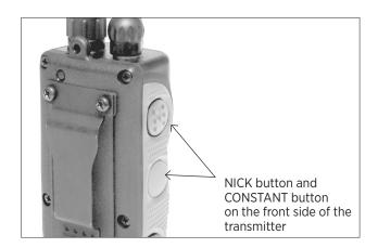
Hold the Nick button and the Constant button on the left side of the transmitter simultaneously down for 3 seconds or until the rapid green blink of the LED on the receiver/collar resumes a slower pace. The code setting work is now completed. If you push the Pager button of the transmitter, the receiver/collar will vibrate.
