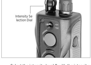
2. Select the intensity level 0 with the intensity selection dial on top of the transmitter.
